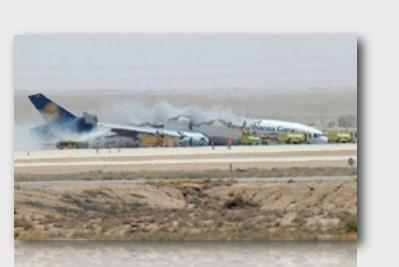
weight, and the MD-11 touched down with a sink rate of 780ft/min - far higher than the typical 120ft/min.
